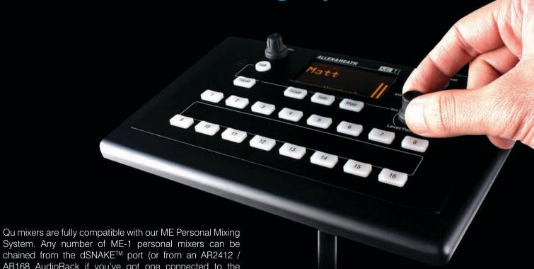
System. Any number of ME-1 personal mixers can be chained from the dSNAKE™ port (or from an AR2412 / AB168 AudioRack if you've got one connected to the dSNAKETM port). Each performer can be given tailored control over their own mix, leaving the engineer free to focus on the audience experience.
