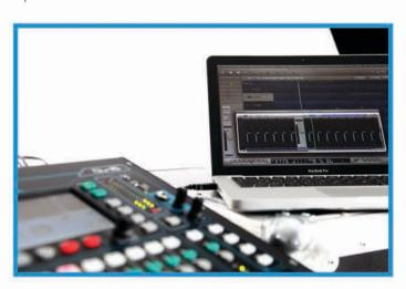
The returns from the computer can be assigned to the Input channels. The interface is class-compliant on Mac OS X – and drivers are available for Windows systems. Either way, it will be recognized straightaway by any DAW supporting ASIO or Core Audio, including Logic, Cubase, Reaper, and Pro Tools.
